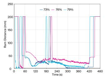
Figure 2. Ram position during mixing of Hi-Sil EZ160G silica compound.
