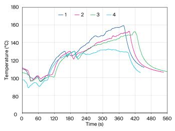
**Figure 5.** Temperature evolution during mixing of *Agilon* 400G compounds.
