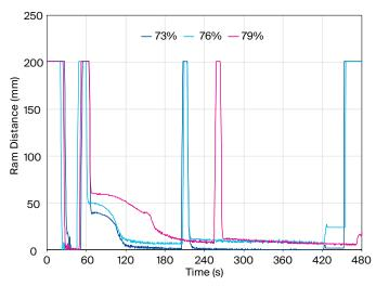
Figure 3. Ram position during mixing of Agilon 400G silica compound.
