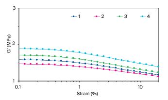
Figure 7. ARES strain sweep at 30°C for *Agilon* 400G silica compounds.
