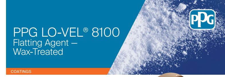
PPG LO-VEL® 8100 flatting agent is high-efficiency flatting agent that is idea for use in a variety of coating systems. *Lo-Vel* 8100 flatting agent is a synthetic amorphous silicon dioxide, wax-treated silica designed for use where a Hegman value of 6 to 6.75 is required. A combination of high flatting efficiency, resistance-to-settling and heat-age stability provides formulation flexibility and expanded process capability.
