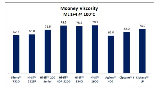
Viscosity at processing temperature shows an increase as silica surface area (reinforcement) increases. Increasing surface area also increases compound stiffness.
