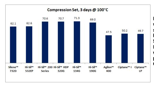
Lower Compression Set was obtained using lower surface area products like Silene™ 732D or Hi-Sil™ 532EP. Lowest set is obtained with silane treated products like Agilon™ or Ciptane™.
