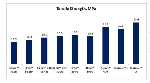
An increase in tensile strength is achieved when using the silane treated products like Agilon™ and Ciptane™.
