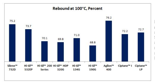
Higher hot rebound is achievable with lower surface area products like Silene™ 732D or Hi-Sil™ 532EP. Even higher hot rebound is obtained with silane treated products like Agilon™ or Ciptane™.
