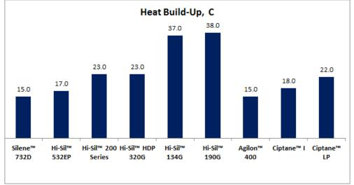
Lower heat build-up is achievable with lower surface area products like Silene™ 732D or Hi-Sil™ 532EP. Theses products provide less stiff compounds compared to the higher surface area products.
